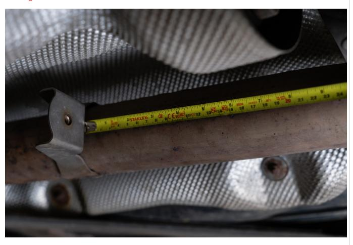
To make it easier to cut the exhaust we recommend removing it from the car. Cut the exhaust 120mm back from the bracket shown above and de-burr the end of the pipe so that the Scorpion pipe is able to slide over it freely.
